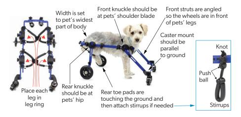
**WIDTH:** Adjust the width in the back from your pet's widest body part(usually the chest). There are several square holes to select from. • Make sure the knobs are tightened and secure.
